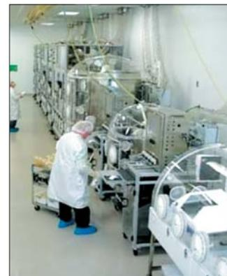
**Figure 2.** An Xcellerex FlexFactory installation for vaccine production. (Source: MediVas)
